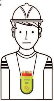
When the V-Watch Personal Voltage Detector is in use with a good working battery, it is always on, always ready to warn of potentially hazardous high voltage. The battery life is approximately six months of continuous use or two years in storage. When the job requiring the protection of the detector for the user is completed, the detector should be closed by pushing down on the top.
